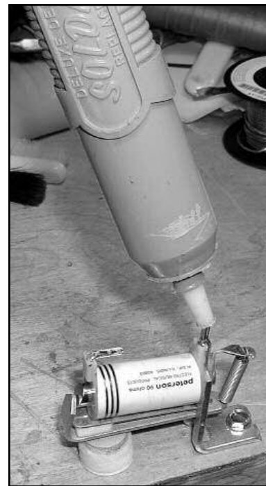
Figure 19. Solder-sucking a Peterson lug to separate it from the coil connection lug.
