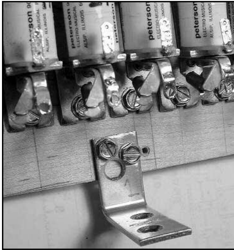
Figure 29. A long plank foot bracket utilizing hand-drilled holes.
