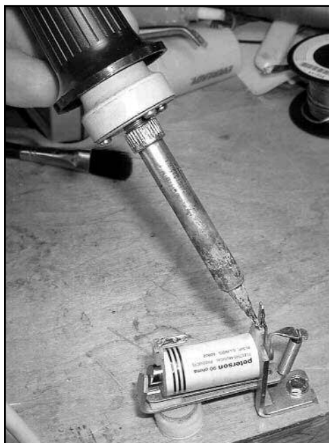
Figure 16. The start of spreading a Peterson valve lug with the soldering iron.
