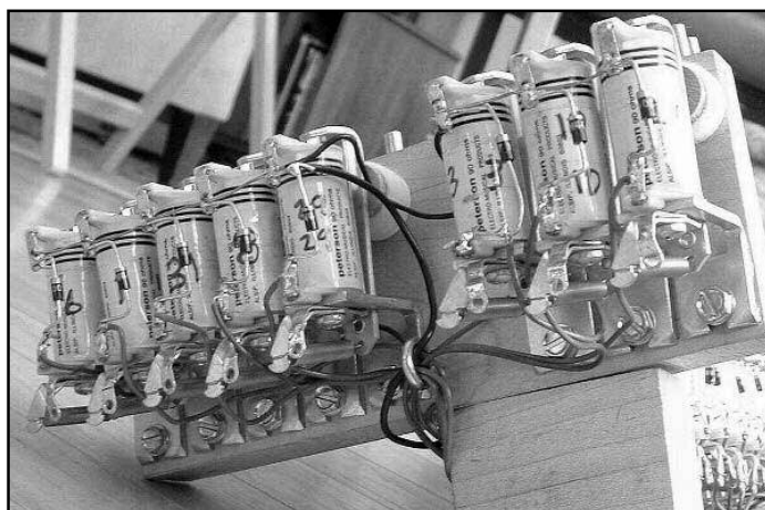
Figure 33. The wiring of the short plank, with screw eyelet guide and the wooden foot.
