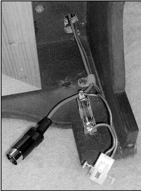
Figure 47. Holes drilled in the bottom of the organ for wiring.
