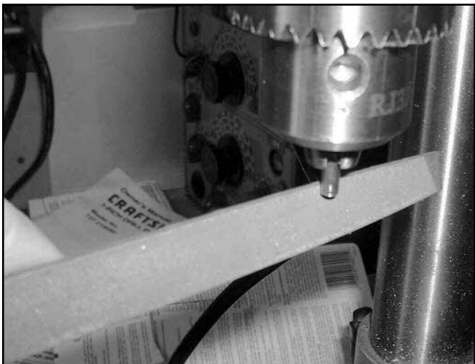
Figure 13. Deburring and beveling the outside edges of the nipple with a file, all the time with the drill spinning.
